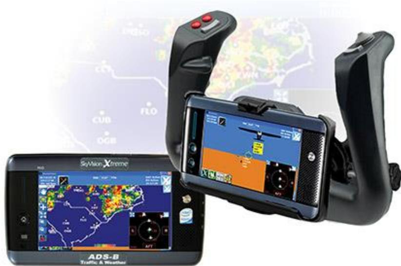
***The portable touch-screen display supports both 1090 ES and 978 MHz modes for ADS-B.***
